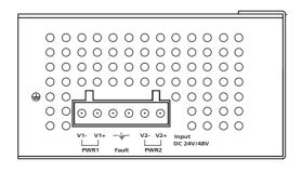
Figure 2-4 Industrial Fast Ethernet Switch upper Panel.
