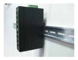
Figure 11: DIN-rail mount industrial device
