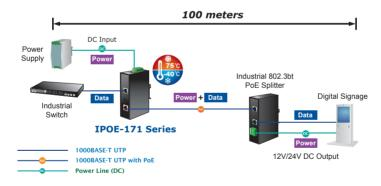
Figure 15: Connected Architecture of IPOE-171-60W and IPOE-171S
