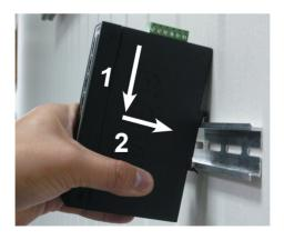
Figure 10: Mounting industrial device on DIN rail.
