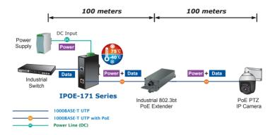
Figure 16: Connected Architecture of IPOE-171-60W and IPOE-E172
