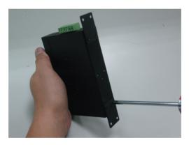
Figure 13: Attach brackets to the industrial device.
