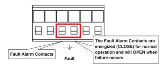
Figure 9: Fault Alarm Contact
